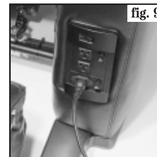
Fig 9. Plug the AC cord into a Grounded Wall Outlet . Turn the Master Switch ON .
