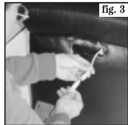
Fig 3. Connect the cord from inside the Seat to the Recline / Calf / Foot Massage Controller , then gently put the cord back in the Seat .
